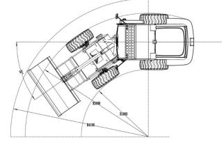
Bucket capacity 0.8m3 Loading capacity1500kgs Max driving Speed 30km/h
